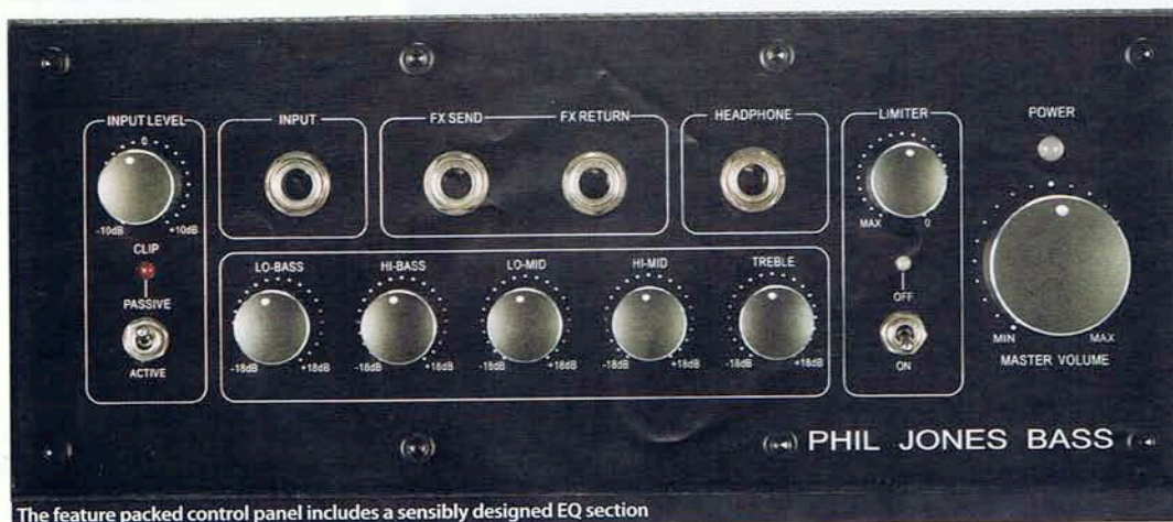
The feature packed control panel includes a sensibly designed EQ section
